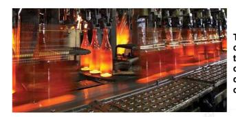
Traditionally Pneumofore supplies glassworks with centralized vacuum systems. Depending on the size of the furnace, also the air compressors of the A Series can be installed to supply the compressed air required during the moulding process of hollow glass containers.
