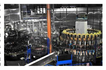
The production of bowls takes place at the blowing machine with double press and transfer station, followed by connecting the stem with the bowl. The productions line allows for so called puled-stem effect: parts of the glass are glued together, then the glass is slightly pulled and the joint is polished. The capacity of the new line reaches up to 65.000 tumbler/day and up to 55.000 stem ware/day.
