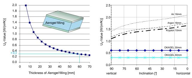
Figure 1: U-value OKAGEL depending on thickness and inclination angle.
