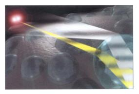
The glass beads have to be partly exposed in order to work properly. The optimum embedment level of the beads in the binder material is 60%. At this level the beads reflect the optimum amount of light back to the driver.
