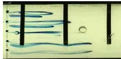
Modelling the effect of the released electric heat on flat, horizontal and vertical electrodes to the glass flow
