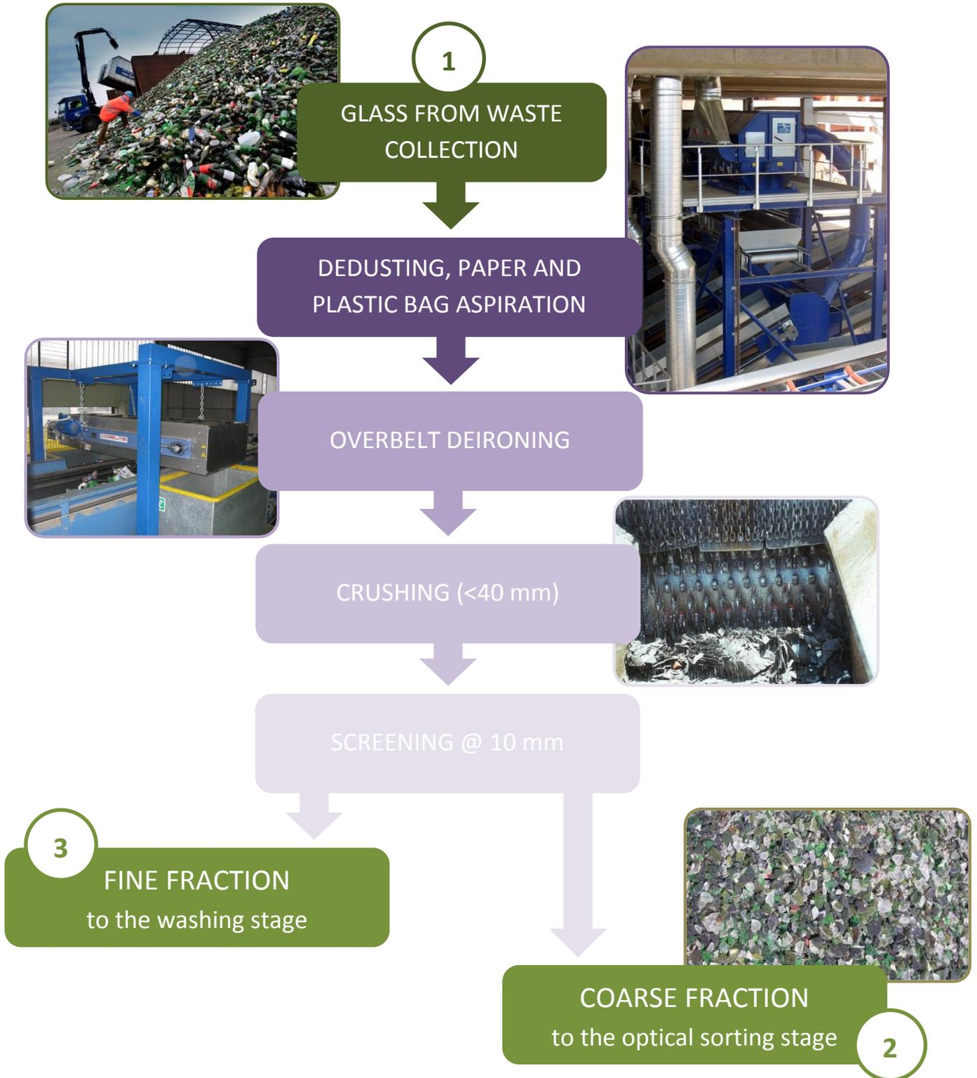
Glass waste recovery - 2<sup>nd</sup> stage: cullet production by optical sorting
