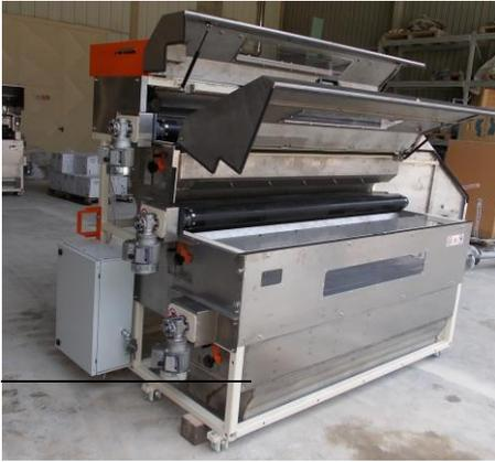
Minerali Industriali uses and provides complete magnetic separation plants. MAG-3 separators have been specially designed by Minerali Industriali to remove main paramagnetic minerals thanks to 3 high field separation stages built in an extremely compact implementation at the same time easily accessible for maintenance.
