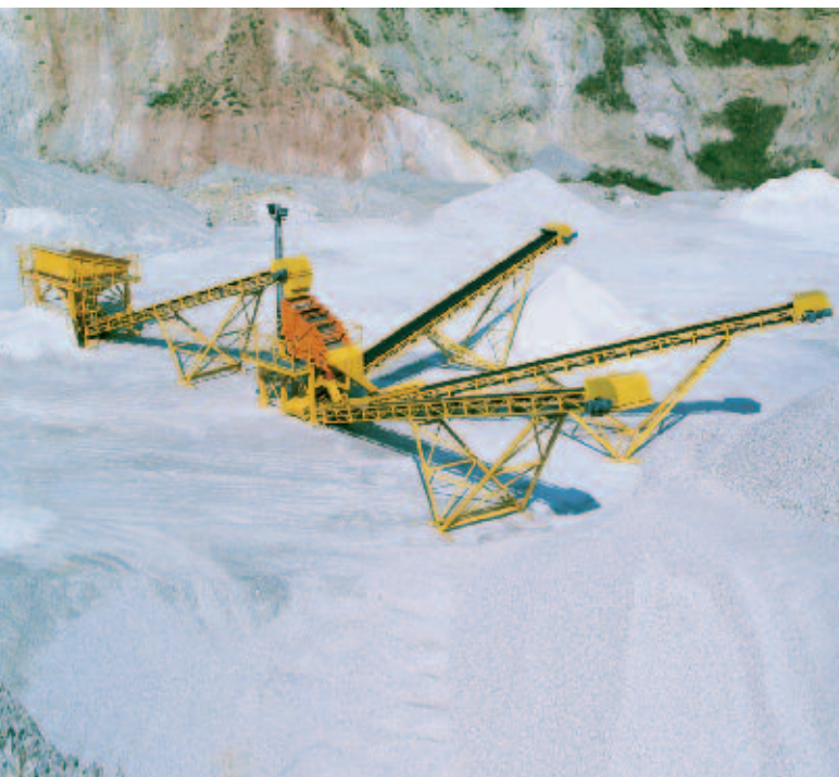
Mogensen Sizer SH 1046 in a short and open design for treatment of broken limestone
