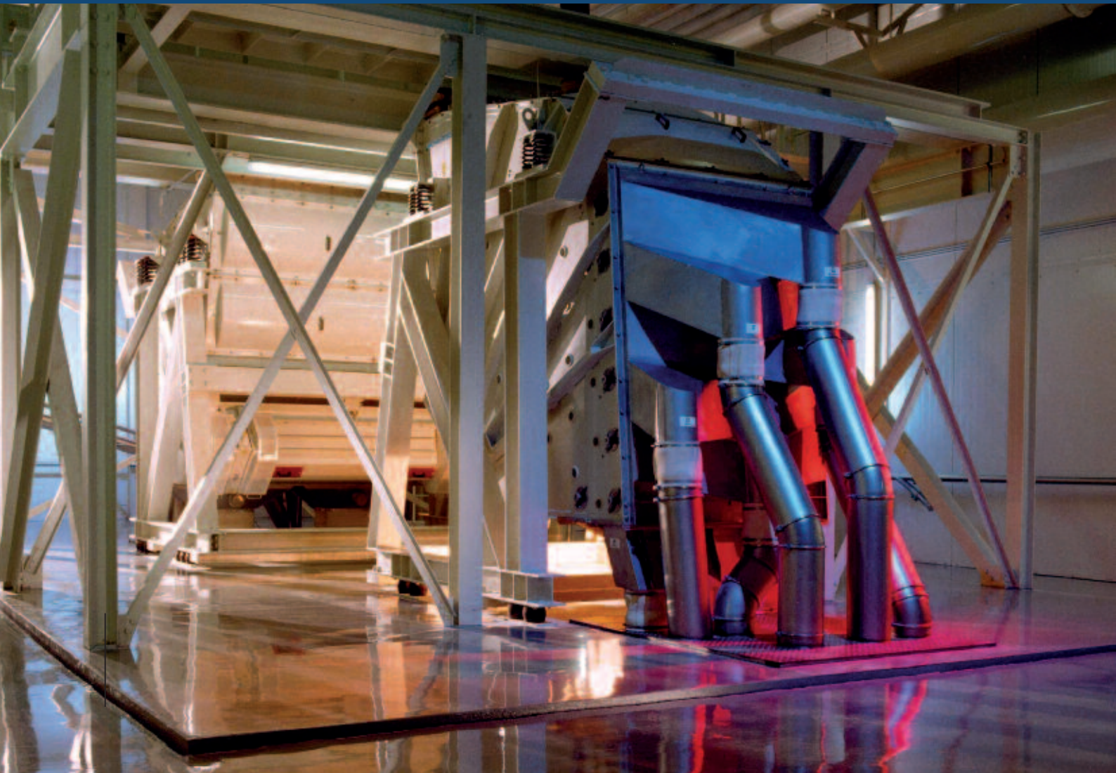
Mogensen Sizer SL 1566 and SL 3068 for screening of white sugar into 6 individual fractions plus scalping of nibs.
