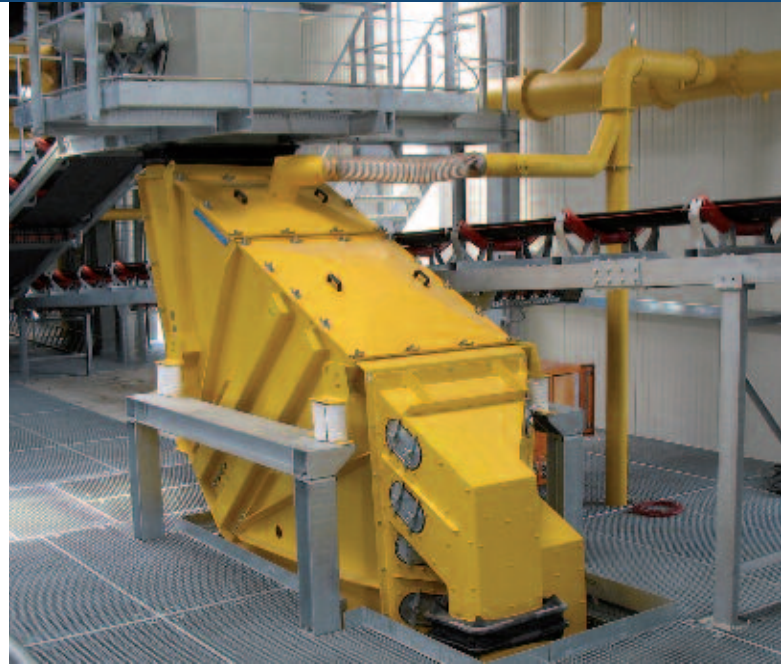
Mogensen Sizer SC 1046 for treatment of broken dolomite in a highly wear-resistant design
