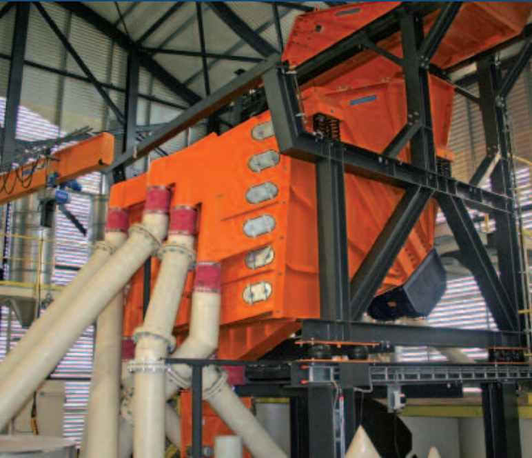
Mogensen Sizer SC 3068 with transverse distribution feeder for treatment of sand for renders and mortars
