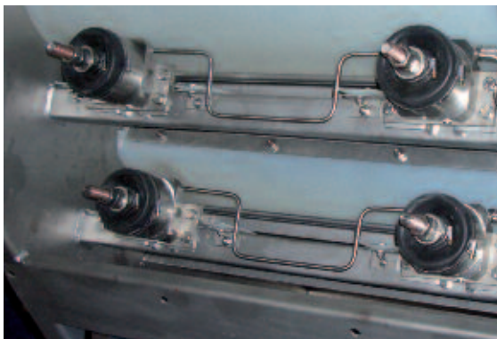
Pneumatic screen cleaning
