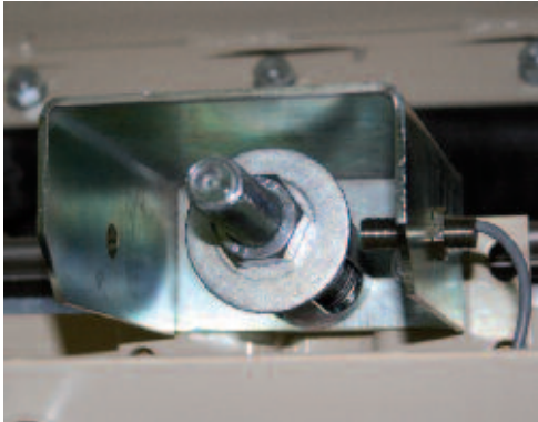
Screen tension monitoring
